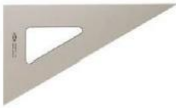
Triangle, for drawing right angles
